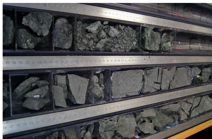
Drilling through fault rock results in many fractured pieces. Photo by Amy West
