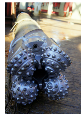
A 'healthy' drill bit: the rotary cone barrel (RCB) used for drilling into hard rock . Photo by Amy West
