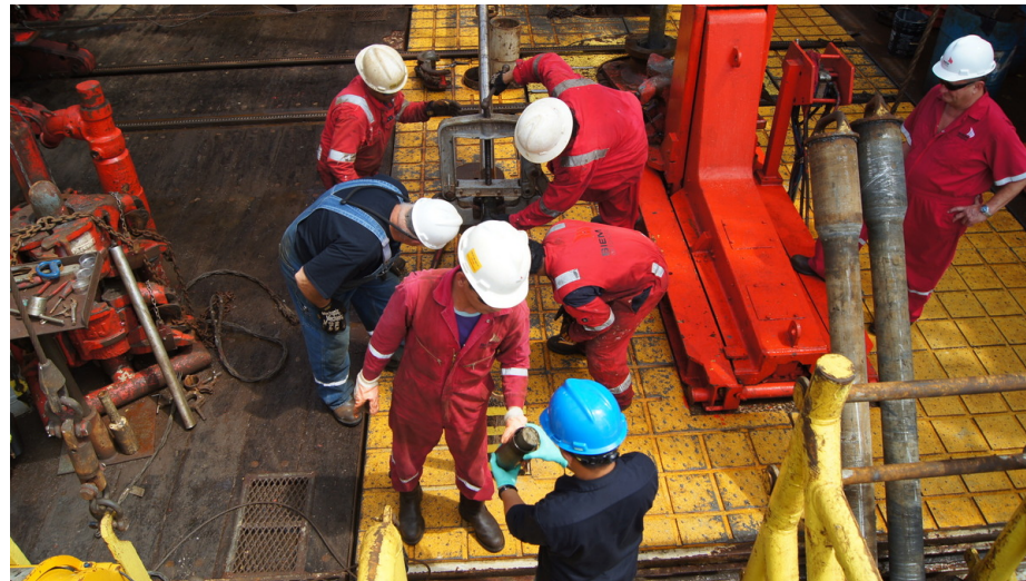
Handing over the first part of the core, “ the core catcher”, which keeps the rest of the core inside the long core barrel as it's pulled to the ship. Photo by Amy West
