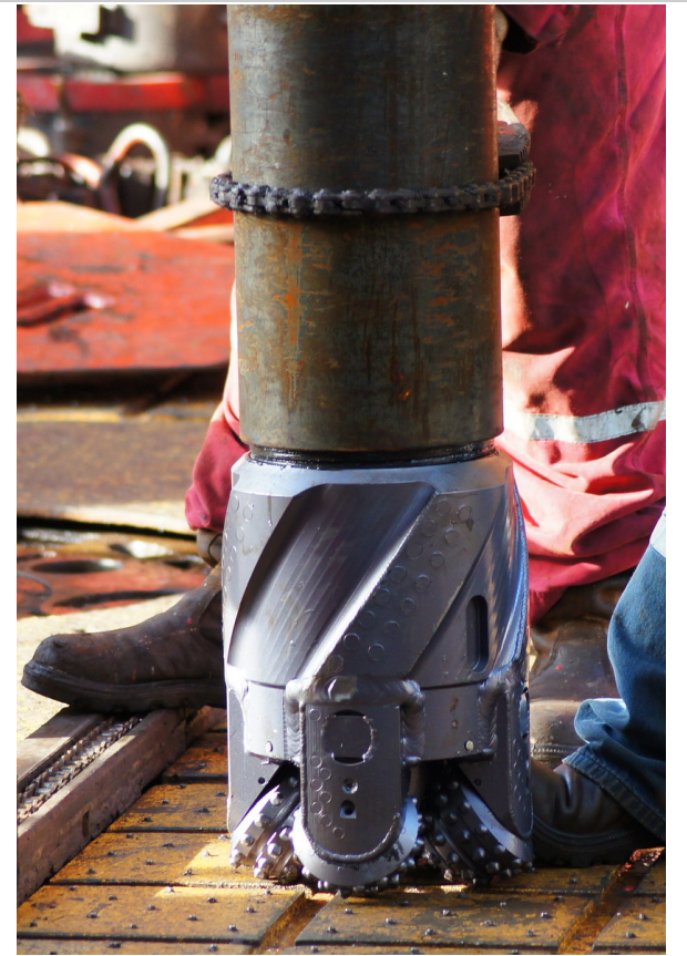
The very end and most important part of the drill pipe: the drill bit. Photo by Amy West
